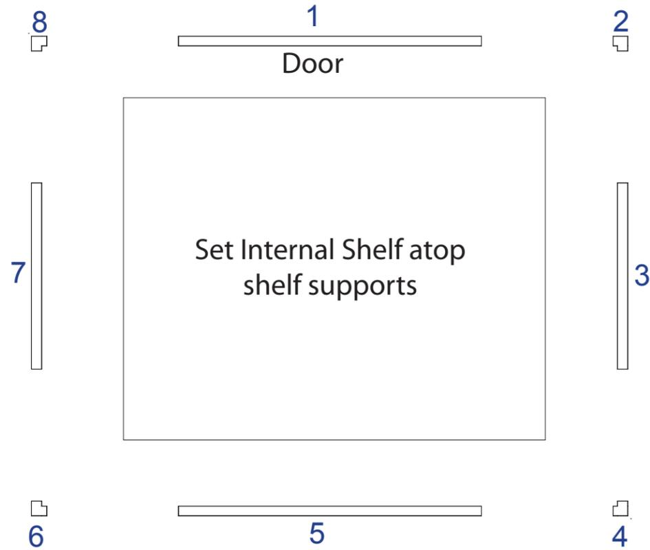
Connect extrusions 1 thru 4 together placing insert as shown in illustration. Then attach hooks to assembled Pedestal.
